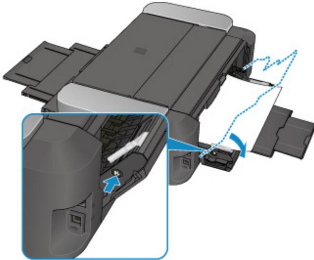
2. Pull the paper out slowly, either from the paper output slot or from the manual feed tray, whichever is easier.
