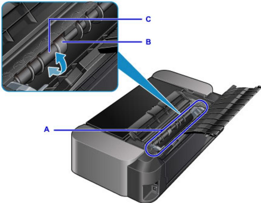
After cleaning the paper feed roller parts with a cotton swab, turn on the power, then clean the paper feed roller from the computer again.
