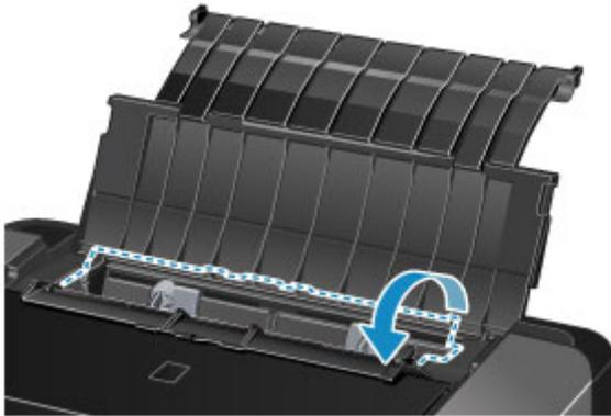
6. Slide the paper guides (E) to open them, and load the paper in the center of the rear tray WITH THE PRINT SIDE FACING YOU.
