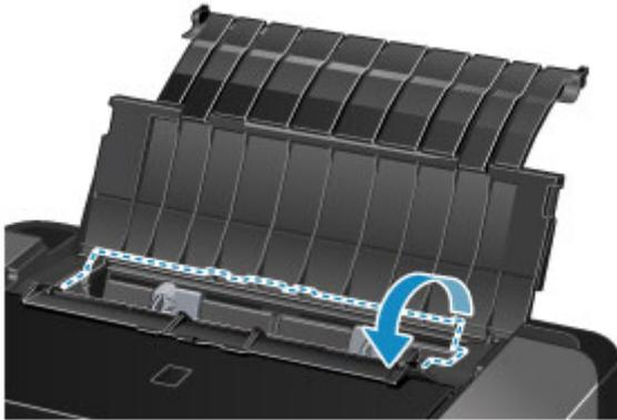
6. Slide the paper guides (E) to open them, and load the envelopes in the center of the rear tray WITH THE ADDRESS SIDE FACING YOU.
