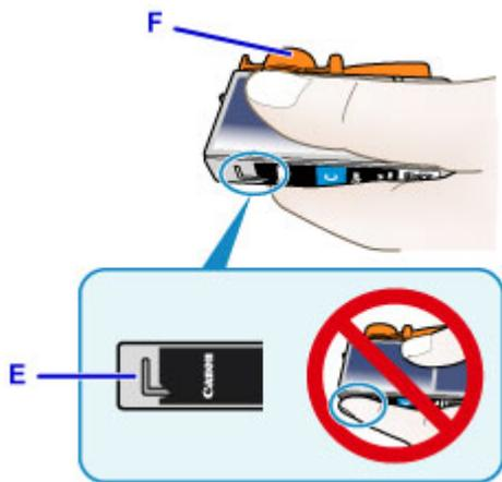
6. Twist the orange protective cap (F) 90 degrees horizontally to remove it off GENTLY.
