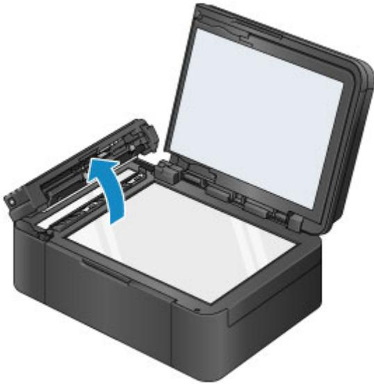
3. With the clean cloth, wipe off any paper dust from the inside of the document feeder cover (A).
