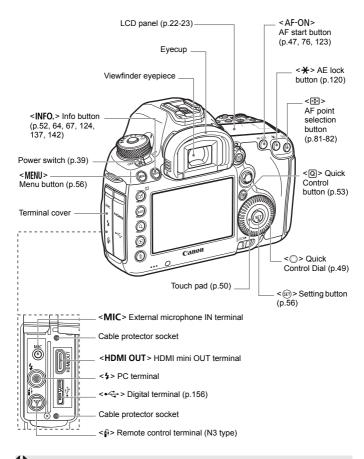
When connecting the interface cable to a digital terminal, you must use the provided cable protector (p.29).
