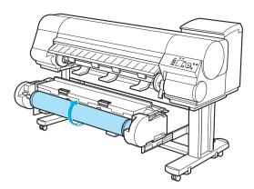
Remove the Roll Holder from the Roll Holder Slot.
