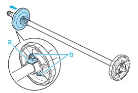
When using a 3-inch paper core, align the tips (a) of 3-Inch Paper Core Attachment #1 with the holes (b) of the Roll Holder and insert it firmly.
