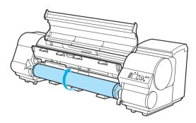
Holding the Roll Holder flange (a), remove the holder from the Roll Holder Slot.
