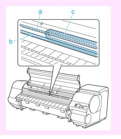
If the Cutter is out, move the Cutter to the right side, away from the paper.
