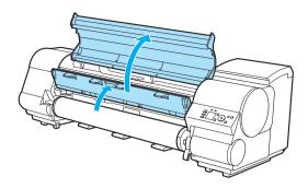
7 Using both hands, rotate the Roll Holder in the direction of the arrow to rewind the roll.
