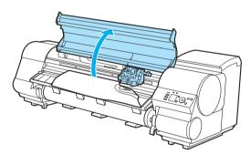
If the Carriage is out, move the Carriage out of the way, away from the paper.
