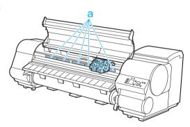
Pull the Printhead Fixer Lever forward all the way to open it completely.
