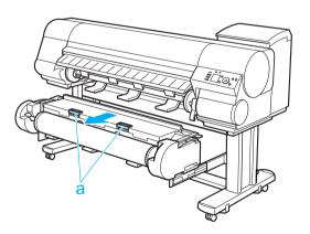
Using both hands, rotate the Roll Holder in the direction of the arrow to rewind the roll.
