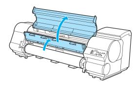
5 Check for paper in the lower part of the printer. Remove any jammed paper here by pushing it to the floor with your fingers.
