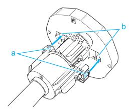
With the edge of the roll paper facing forward as shown, insert the Roll Holder from the right of the roll. Insert it firmly until the roll touches the flange (a) of the Roll Holder.
