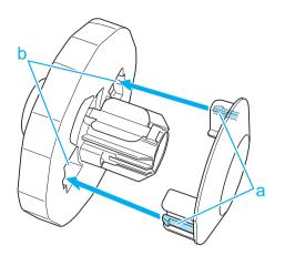
Insert the Holder Stopper from the left in the Roll Holder as shown. Holding it at the position shown (b), push it firmly in until the flange (a) of the Holder Stopper touches the roll. Lock the Holder Stopper lever (c) by pushing it down toward the shaft side.
