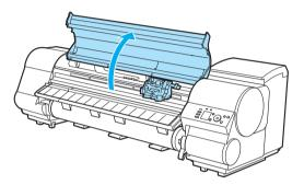
If the Printhead Fixer Cover or Printhead Fixer Lever is dirty, use a damp cloth that you have wrung out completely to wipe it clean.
