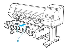
Holding the Roll Holder so that the side with the white gear faces the side of the Roll Holder Slot with a white gear, load the Roll Holder shaft (a) into the grooves (b) on both ends of the Roll Holder Slot.
