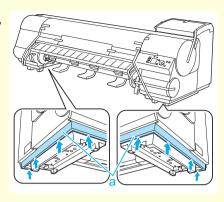
Remove tape and packaging material attached to the printer. Also open the Top Cover and remove stoppers and spacers inside the printer.
