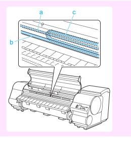
If the ventilation duct (a) is dirty, use a damp cloth that you have wrung out completely to wipe it clean. Move the Carriage out of the way manually if the Carriage is concealing the ventilation duct, and then clean the duct.
