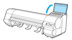
Lift the stopper (a) of the lnk Tank Lock Lever (a). Lift the lnk Tank Lock Lever until it stops, and then push it down to the front.
