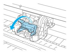
Pull up the Printhead Fixer Cover to open it completely.
