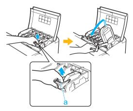
Hold the Ink Tank by the handle (a) and remove it.
