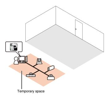
Before installing the camera in the final location, set the camera in a temporary space to carry out the initial settings. Connect the cameras to the same network as the computer.
