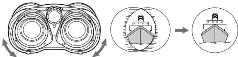
Look through the binoculars and adjust the width until the left and right images converge as shown above.
