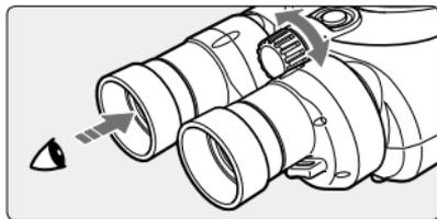
First look through the left eyepiece only and adjust the focusing knob until the object looks sharp.
