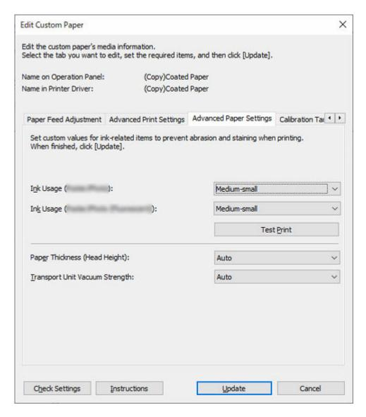
Determines and sets the ink level that is expected to produce no bleeding or grazing of ink and produce the best test print results when viewed.
