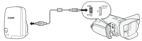
When connecting the GP-E2 GPS Receiver to the camcorder, use the connecting cable supplied with the receiver.
