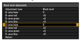
Adjust [D-area base] to lighten the black level, and adjust [Red], [Green], and [Blue] to obtain an optimal black level color tone, as needed.
