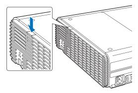
As you hold down the lamp cover release button, slide the lamp cover toward the back, and then lift the cover to open it.
