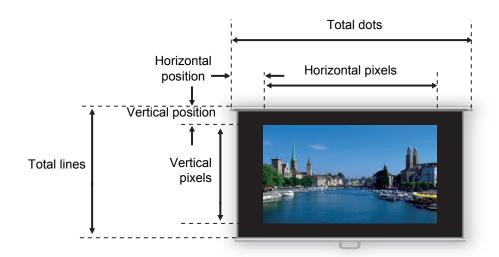
Perform this adjustment if the Auto PC function (P76) or the Input signal select function (P76) cannot adjust the projected image correctly.
