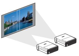
Blend the overlapping edges of images from multiple projectors to make the overall image more seamless. (P159)
