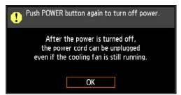
2 When this window is displayed, press the POWER button again to turn off the power.
