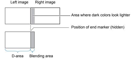
Here, the non-overlapping image area (from the end marker toward the center of the image) is called area "D."
