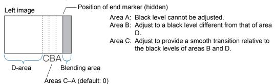
When the projected image has multiple blending areas (on the top, bottom, and each side), the width of areas A, B, and C must be adjusted to suit these blending areas.
