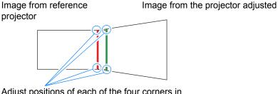
Adjust positions of each of the four corners in the overlapping area. Correcting the position of one point will also move the point on the opposite side of the overlapping area, so that the screen as a whole is corrected.
