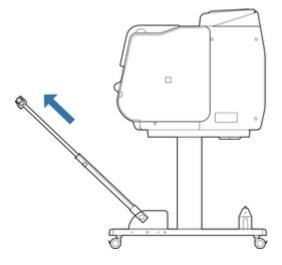
• When lengthening the basket arm, first return the basket to an unwound state while pressing the basket rewind button on the right edge of the basket rod (tag side), and then make the change.
