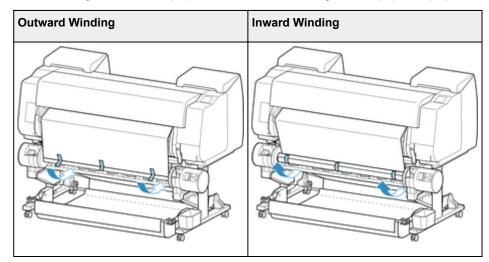
4. While making sure that roll paper is flat, secure left edge of roll paper to paper core with tape.
