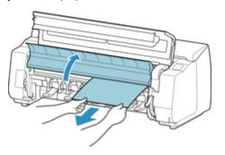
After removing the paper, inspect the interior to ensure paper fragments or other objects do not remain, and lower the output guide.
