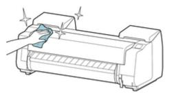
• Open top cover and output guide and clean parts that come in contact with paper (A, B).
