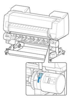
7. Hold flanges (A) so that roll holder's white gear is on left, align roll holder shaft with roll holder slot left and right guide grooves (B), and load.
