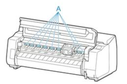
4. While pressing button (A) in center of print head lock lever, pull it forward to open it until it stops.
