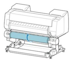
6. Change **Roll Holder Lock** switch on roll unit to release position.
