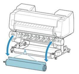
10. Push holder stopper lever (A) toward shaft to release lock, and while holding in position (B), remove holder stopper from roll holder.
