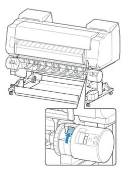
5. Hold flanges (A) so that roll holder's white gear is on left, align roll holder shaft with roll holder slot left and right guide grooves (B), and load.
