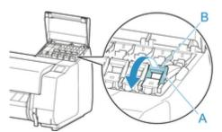
3. Lift ink tank lock lever until it stops, and then push it down toward front.
