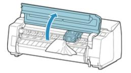
3. If the Carriage is out, move the Carriage out of the way, away from the paper.
