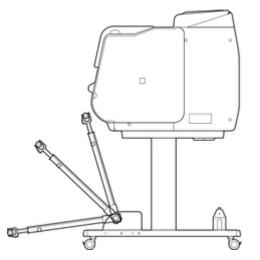
When securing the basket arm, attach the basket locking support to the basket arm (A) on both sides.
