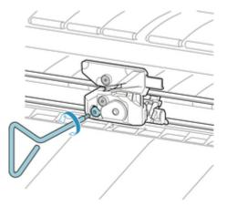
4. Remove cutter blade while holding A.
