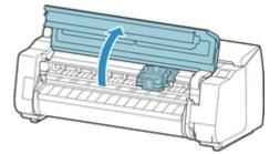
2. If the print head locking cover and print head lock lever are dirty, use a damp cloth that you have wrung out completely to wipe them clean.
