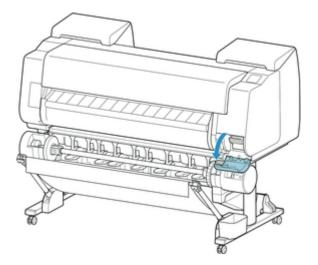
3. Hold the used maintenance cartridge by the grip (A) with one hand and put your other hand under the maintenance cartridge to hold it firmly on the bottom, keeping it level as you pull it out.
