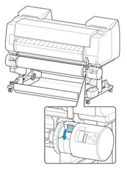
7. Change feed flap switch on top of roll unit to feed icon position on the left.
