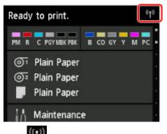
If the icon is not displayed, follow the procedure below to enable wireless LAN and to connect the printer to the wireless router.
