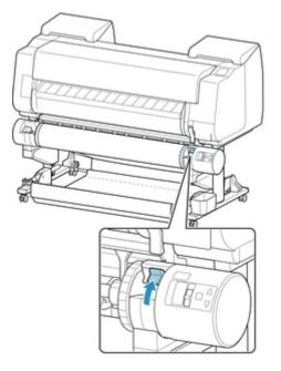
9. Hold roll holder by its flanges (A), and remove from roll unit.
