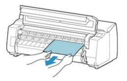
6. If you cannot see the paper, lift the output guide, remove the roll holder, and remove the jammed paper from underneath.
