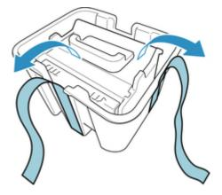
9. Lift print head by blue handle and remove orange protective cap (2).
