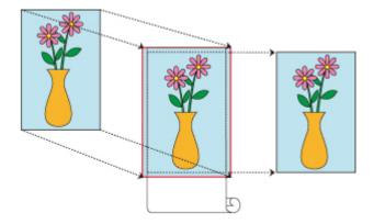
Procedure for printing borderless (without white margins around the edges) by enlarging/reducing documents to match roll paper width.
