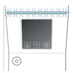
If the **Status** lamp is flashing orange, check the message on the touch screen and take action as necessary.
