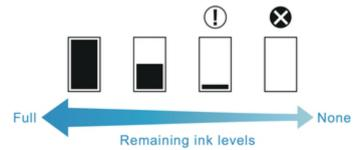
If the touch screen indicates to replace the ink tank, replace the ink tank. If a message is displayed indicating to check the remaining ink levels, or after tasks that consume a lot of ink such as large-format printing or head cleaning, check the remaining levels and replace ink tank as needed.
