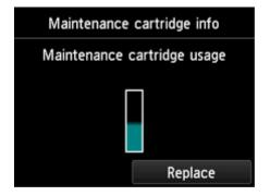
If the touch screen indicates to replace the maintenance cartridge, replace the maintenance cartridge. If a message appears indicating to check the remaining capacity of the maintenance cartridge, or before tasks that deplete much of the capacity such as head cleaning or preparations to move the printer, check the remaining maintenance cartridge capacity and prepare a new maintenance cartridge as needed.
