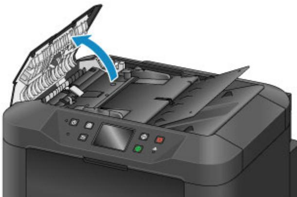
3. Use the cloth to wipe off any paper dust inside the document feeder cover (A).
