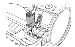
If the ink tank does not fit in the holder, make sure the color of the ink tank lock lever matches the color of the ink tank, and check the orientation of the ink tank. 8
