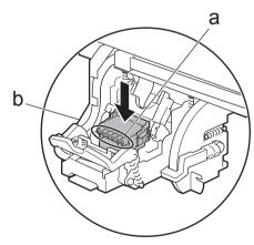
Pull the printhead fixer cover down toward the front to lock the printhead in place.
