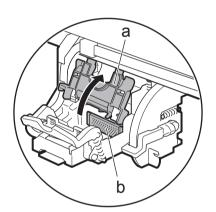
Hold the printhead by the grips (a) as you remove it from the pouch.
