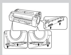
The way to set the printer down or to carry with the load only to the center of the printer, may cause damage to the printer.
