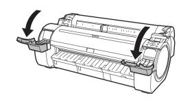
While pressing the stopper of the ink tank lock lever inwards, open the ink tank lock lever upwards.
