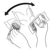
• Failure to shake ink tanks may result in reduced print quality because ink ingredients have settled on the bottom
