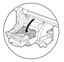
Push the printhead fixer lever all the way back.
