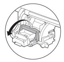
Lift the printhead fixer cover (a) to open it fully.
