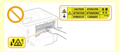
Do not carry the machine with the paper drawer or optional paper feeder installed. Otherwise, they may fall, resulting in injury.
