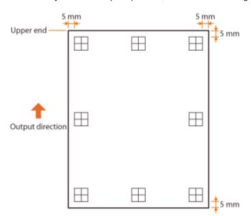
The size of the mark " for checking the print position is as shown in the illustration below.
