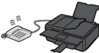
The printer will receive the fax automatically when the fax ring pattern is detected.
