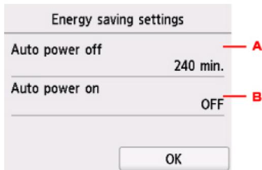
A. Specify the length of time to turn the printer off automatically when no operation is made or no printing data is sent to the printer.
