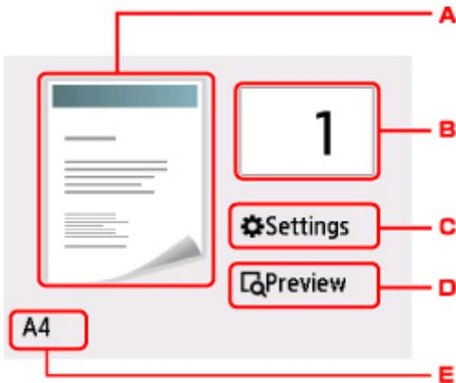
A. The scanning method and copy layout are displayed.
