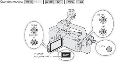
1 <u>Physical buttons</u>: Press the MENU button and, while holding it pressed down, press the assignable button whose function you wish to change.
