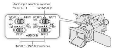
1 Select the INPUT terminals as the audio input for the desired audio channel.
