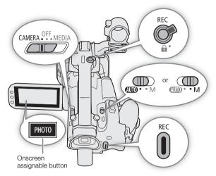
• You can also press the REC button on the handle unit or the START/STOP button on the supplied wireless controller.
