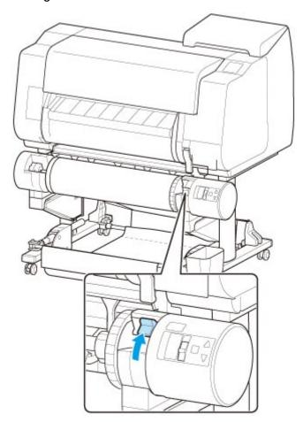
7. Hold roll holder by its flanges (A) and remove from roll holder slot.
