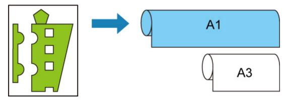
When the A1 width roll paper is loaded on the upper roll, A3 width roll paper on the lower, and the paper source can be switched, and when an A4 size image is enlarged by 160 % specified in **Scaling** on **Enlarge/Reduce**, the A1 width roll paper is selected, as the image width exceeds that of A3.
