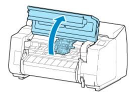
7. If the print head locking cover and print head lock lever are dirty, use a damp cloth that you have wrung out completely to wipe them clean.
