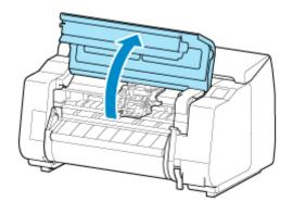
6. Align the angle adjustment lever with the red square and close the top cover.
