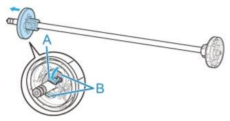
2. If using 3-inch core paper, align 3-Inch Paper Core Attachment tabs (A) with Roll Holder holes (B) and insert firmly.
