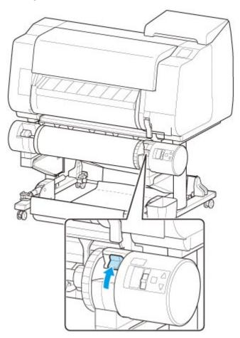
9. Hold roll holder by its flanges (A), and remove from roll unit.
