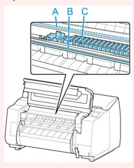
8. If ventilation duct (A) is dirty, use damp cloth that you have wrung out completely to wipe it clean.
