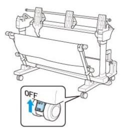
2. Move the stacker to front of the printer with the stand, and then push in the convex portions (A) on both sides of the foot of the stacker until they hit the stand of the printer.
