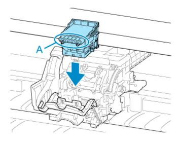
15. Lower print head locking cover to front and lock print head.
