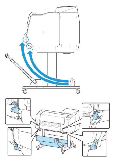
• When attaching the basket rod (cord side) to the front of the printer, make sure both ends of the rod (A) are securely hooked onto the attachment parts.
