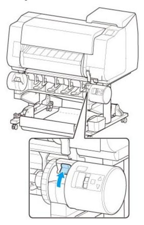
3. Hold flanges (A) so that roll holder's white gear is on left, align roll holder shaft with roll holder slot left and right guide grooves (B), and load.
