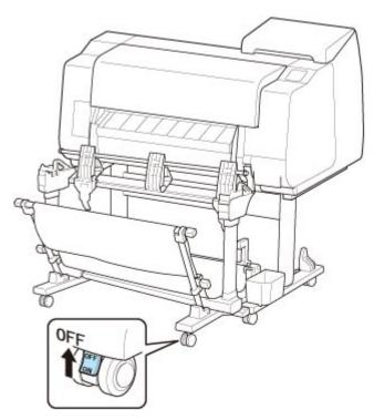
2. Pull out the stacker toward you to remove the stacker from the printer.
