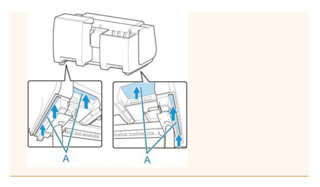
2. Remove tape and packaging material attached to the printer. Also open the top cover and remove stoppers and spacers inside the printer.
