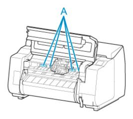
9. Pull down print head lock lever toward the front while holding its center (A) with your fingertip.
