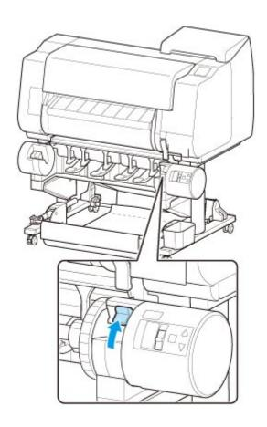
7. Hold flanges (A) so that roll holder's white gear is on left, align roll holder shaft with roll holder slot left and right guide grooves (B), and load.
