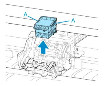
• Never touch the metal contacts of the carriage. Furthermore, do not allow any dirt or debris to become adhered to the metal contacts of the carriage. These may damage the printer.
