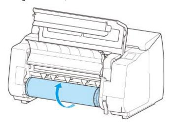
7. Hold Roll Holder by its flanges (A) and remove from roll holder slot.
