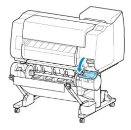
6. Hold the used maintenance cartridge by the grip (A) with one hand and put your other hand under the maintenance cartridge to hold it firmly on the bottom, keeping it level as you pull it out.
