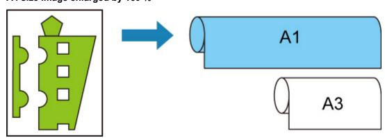
When the A1 width roll paper is loaded on the upper roll, A3 width roll paper on the lower, and the paper source can be switched, and when an A4 size image is enlarged by 160 % specified in **Scaling** on **Enlarge/Reduce**, the A1 width roll paper is selected, as the image width exceeds that of A3.
