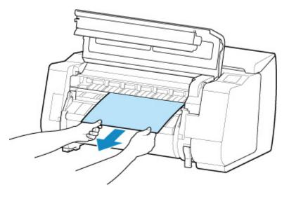
After removing the paper, inspect the interior to ensure paper fragments or other objects do not remain.
