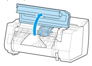
3. If the Carriage is out, move the Carriage out of the way, away from the paper.
