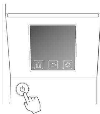
When startup is finished, **ON** button lights up, and printer enters standby mode.
