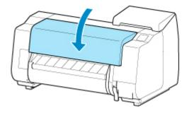
5. Tape down printer covers to secure them, in the reverse order of tape removal during installation.
