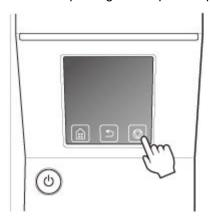
When you press the **Stop** button during printing, the printer operation varies depending on the current status.
