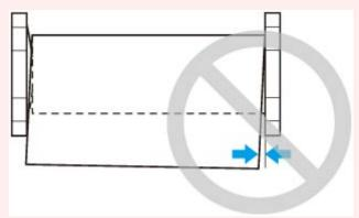
• Depending on the paper, the roll paper may be scratched when being fed and not feed well. In this case, you must feed the paper manually after setting **Paper retention setting** to **Release** on the touch screen. Lift the release lever, advance the roll paper until its leading edge appears on platen, lower the release lever, and then proceed to the next step. However, if
