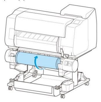
Apply adhesive tape to the rewound paper to hold it in place, if necessary.
