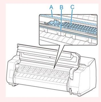
3. Place cut sheet with the print side up, insert in portrait orientation between platen (A) and paper retainer (B), and align paper's far edge using the following steps.
