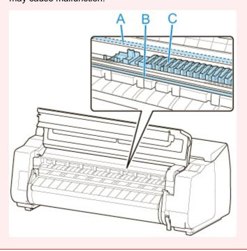
8. If ventilation duct (A) is dirty, use damp cloth that you have wrung out completely to wipe it clean.
