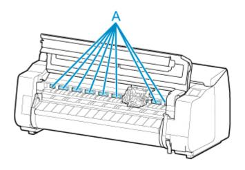
9. Pull down print head lock lever toward the front while holding its center (A) with your fingertip.
