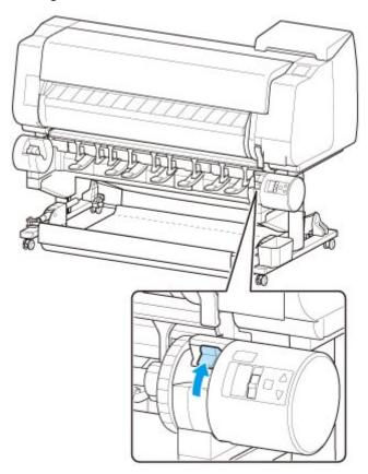
3. Hold flanges (A) so that roll holder's white gear is on left, align roll holder shaft with roll holder slot left and right guide grooves (B), and load.
