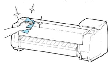
• Open the top cover and output guide and clean parts that come in contact with paper (A, B) and sensor (C).
