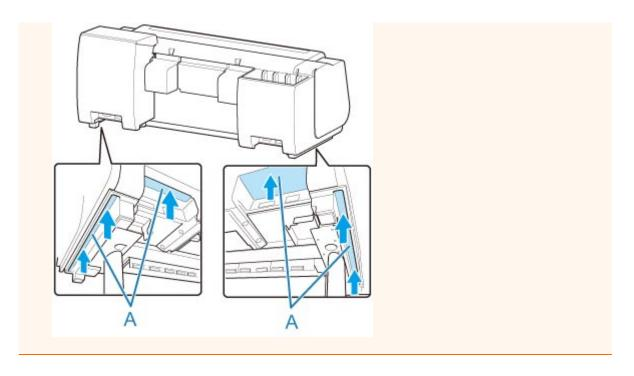
2. Remove tape and packaging material attached to the printer. Also open the top cover and remove stoppers and spacers inside the printer.
