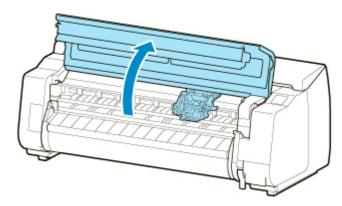
7. If the print head locking cover and print head lock lever are dirty, use a damp cloth that you have wrung out completely to wipe them clean.
