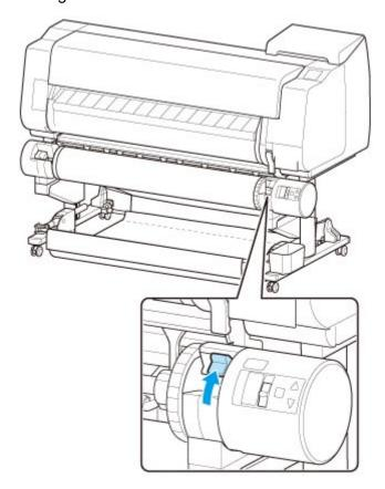
7. Hold roll holder by its flanges (A) and remove from roll holder slot.
