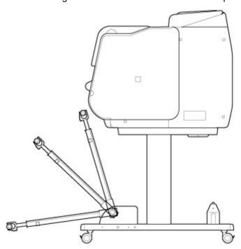
When securing the basket arm, attach the basket locking support to the basket arms (A) on both sides.
