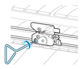
7. Remove cutter blade while holding A.
