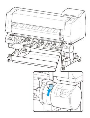
7. Hold flanges (A) so that roll holder's white gear is on left, align roll holder shaft with roll holder slot left and right guide grooves (B), and load.
