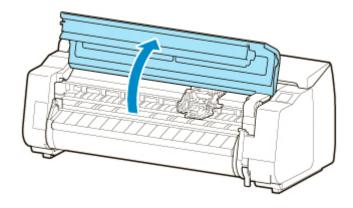
6. Align the angle adjustment lever with the red square and close the top cover.
