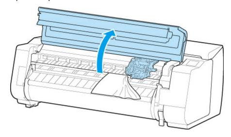
3. If the Carriage is out, move the Carriage out of the way, away from the paper.
