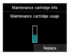
If the touch screen indicates to replace the maintenance cartridge, replace the maintenance cartridge.
