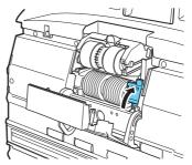
**9** Close the roller cover. Make sure that the front unit is completely closed by pushing until you hear a click.
