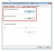
The number of sheets fed by the feed rollers or separation pads is reset.
