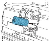
Put the feed roller in place (1), and align the notch in the roller's axle with the shaft on the scanner (2).
