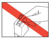
Install the new cartridge with the nozzles facing to the right.
