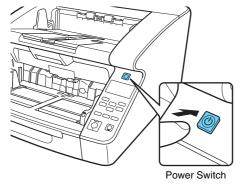
The power button lights green when the power turns ON.
