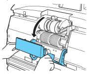
3 Pull the roller lock lever down.
