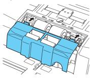
Push the front of the retard roller cover in. Make sure that the front unit is completely closed by pushing until you hear a click.
