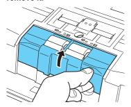
3 Push the roller lock lever up (1) and move it to the left (2) to unlock the roller.
