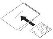
5 Load the document with the sealed end of the carrier sheet as the leading edge.
