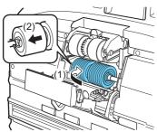
8 Push the roller lock lever up to lock the feed roller.
