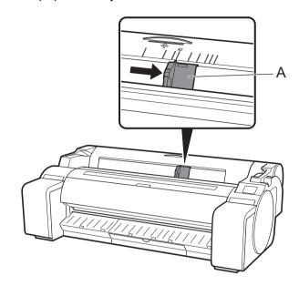
Prepare 1 sheet of paper for adjustment. Identify the printed side by referring to the bag in which the paper came.
