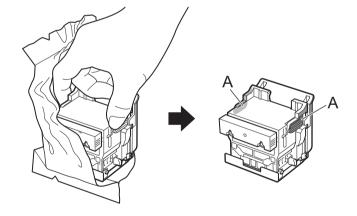
Remove the orange protective cap (A), and then remove the other orange protective cap (B) by holding the tab part (C).
