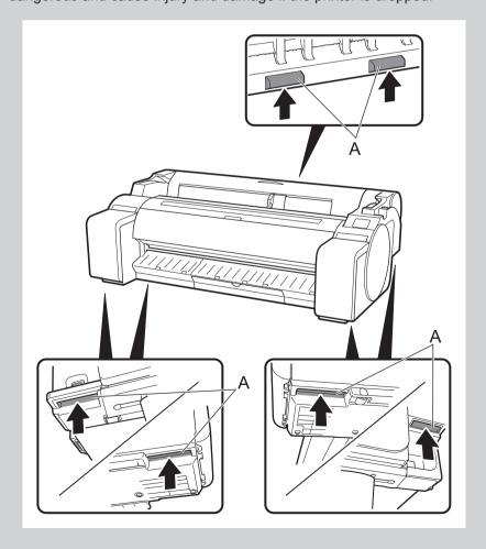
Caution • When setting the printer down temporarily make sure to put the printer on a flat, stable surface.
