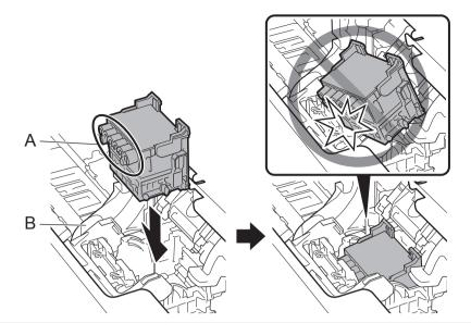
Pull the print head locking cover down toward the front to lock the print head in place.
