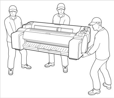
• When moving the printer, firmly grasp the carrying handles (A) under each side and at the rear side. Holding the printer at other positions is dangerous and cause injury and damage if the printer is dropped.
