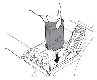
0 **Important**   If the ink tank does not fit into the holder, check that the color on the ink tank label matches the color shown on the ink tank lock lever. Check also the orientation of the ink
