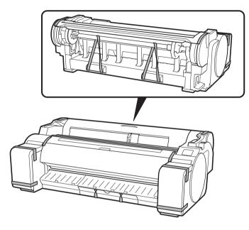
Have 3 people lift up the printer. Have 1 person grasp the carrying handles at the bottom of each side, and 1 person grasp the handles in the middle of the rear side.
