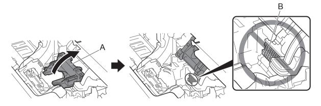
Remove the print head from the bag by holding the tab parts (A).
