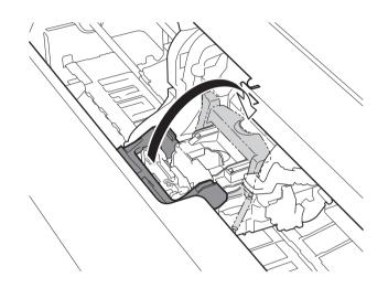
Check that the angle adjustment lever is aligned with the position of the red ■ (A). If it is not aligned, align the angle adjustment lever with the red ■ (A).
