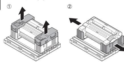
Remove all of the tape and other packaging material. Remove the tape affixed to the roll holder.
