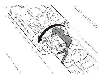
Open the print head locking cover (A) and select **OK** on the touch screen. At this time, check that there is no dirt on the electrical contacts (B) of the carriage.
