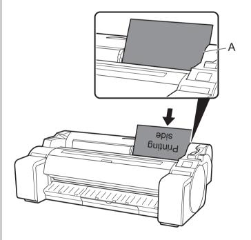
Adjust the position of the width guide (A) according to the size of the loaded paper. Align the width guide exactly with the paper to avoid the loaded paper from tilting or crinkling.
