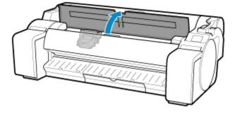
6. Align the angle adjustment lever with the red square and close the top cover.
