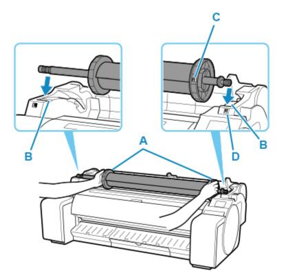
**5.** Holding the roll holder flange (A), guide the holder along the slide guides (b) on both ends, keeping the holder level as you load it in the roll holder slot.
