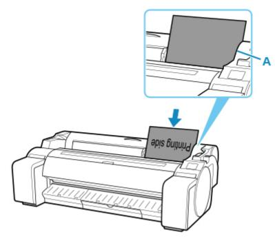
**4.** Move the width guide (A) carefully to match the size of paper loaded.
