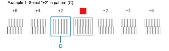
Example 2: Move the angle adjustment lever to a position between the numbers or between the number and the square (D) of the two sets of lines that are least misaligned. In this case, select -1.
