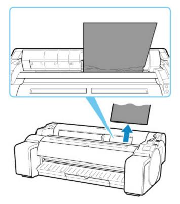
• If the paper is jammed by the ejection guide
