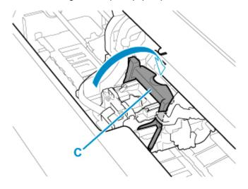
**14.** Align angle adjustment lever with the red square position.
