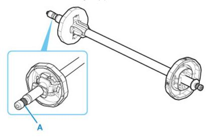
When the noise starts, clean the gear with the following procedure.
