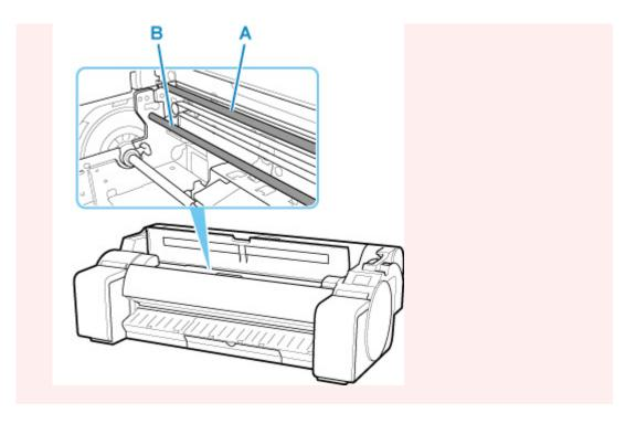
If the paper from a roll is jammed by the paper feed slot
