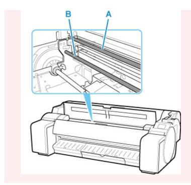
If the paper from a roll is jammed by the paper feed slot Remove the jammed paper from the paper feed slot.
