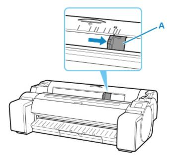
**3.** Load a single sheet printing-side up in the feed slot, with the right edge aligned with the paper alignment line (A) to the right of the roll paper cover.
