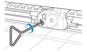
6. Remove cutter blade while holding A.
