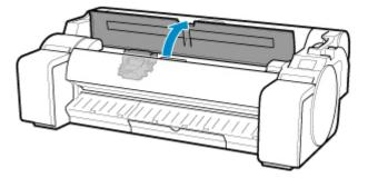
**5.** If the print head locking cover and print head lock lever are dirty, use a damp cloth that you have wrung out completely to wipe them clean.
