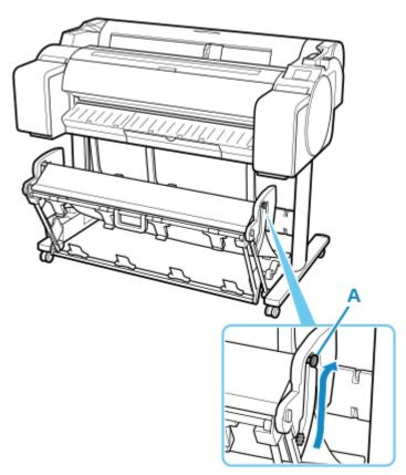
When using 24-inch or A1 (portrait) roll paper, pull out the Adjustable Stopper (A). This completes the procedure for switching to Extended position A.
