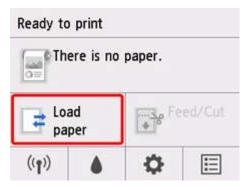
2. Tap Load cut sheet or Replace cut sheet.
