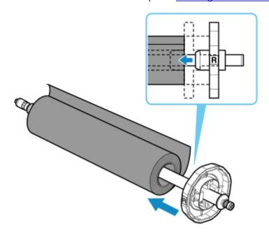
3. Load the Roll Media in the printer. (See "Loading Rolls in the Printer")
