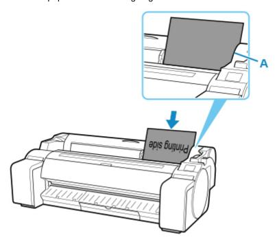
**4.** Move the width guide (A) carefully to match the size of paper loaded.
