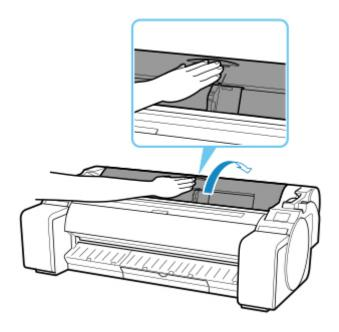
**5.** Using both hands, rotate the roll holder toward the back to rewind the roll.
