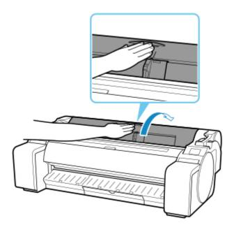
**4.** Holding the roll holder flange (A), rest the roll holder shaft on the roll holder resting ledge (B).
