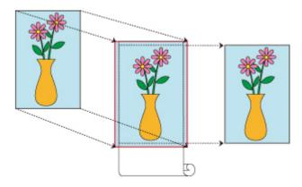
Procedure for printing borderless (without white margins around the edges) by enlarging/reducing documents to match roll paper width.
