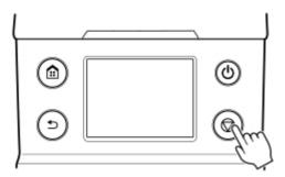
When you press the **Stop** button during printing, the printer operation varies depending on the current status.
