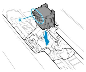
12. Grasp tab (D) of print head locking cover and lower it to front to lock print head.
