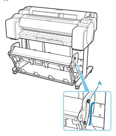
2. When using 24-inch or A1 (portrait) roll paper, pull out the Adjustable Stopper (A).
