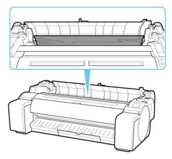
• If the paper is jammed by the ejection guide
