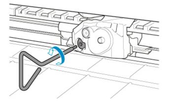
6. Remove cutter blade while holding A.
