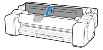
**5.** If the print head locking cover and print head lock lever are dirty, use a damp cloth that you have wrung out completely to wipe them clean.
