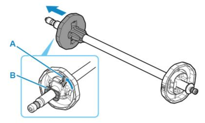
If using 3-inch core paper, align 3-inch paper core attachment tabs (A) with roll holder holes (B) and insert firmly.
