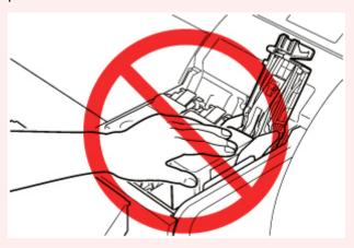
• If a 4.4 fl oz (130 ml) ink tank is installed facing the wrong direction, the rotating part of the ink tank lock lever come out of place. If this happens, open the ink tank lock lever to return it to the proper position.
