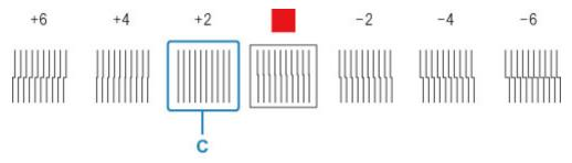
Example 2: Move the angle adjustment lever to a position between the numbers or between the number and the square (D) of the two sets of lines that are least misaligned. In this case, select -1.
