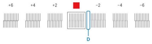
**8.** Open top cover and move angle adjustment lever to match number (or square) of straightest set of lines.
