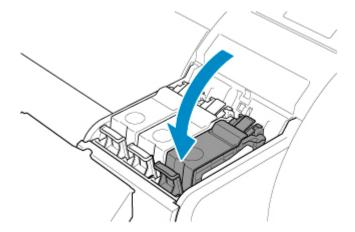
• Do not push the ink tank in by hand. Forcing the ink tank into the holder may damage the printer.
