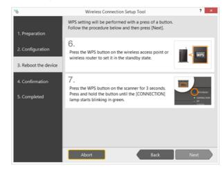
(6) Press the WPS button on the access point to activate the connectionwaiting state.
