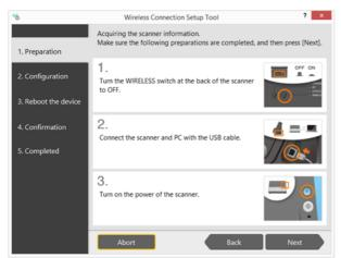
(1) Turn off the WIRELESS switch on the rear of the scanner.
