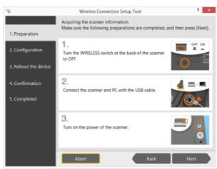
(1) Turn off the WIRELESS switch on the rear of the scanner.
