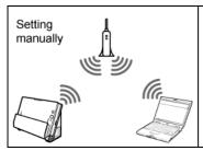
If the access point does not supports the WPS function, make the access point settings manually to establish connections.
