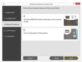
(4) Turn on the WIRELESS switch on the rear of the scanner.
