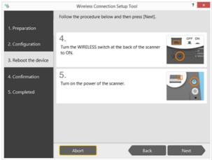
(4) Turn on the WIRELESS switch on the rear of the scanner.
