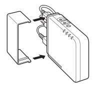
You can attach the stand to set the device upright. In addition, placing the scanner on the stand will stabilize the device.
