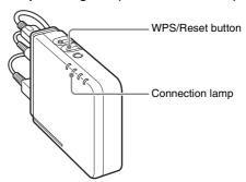
The device communicates with the waiting access point to acquire and automatically configure the required Wi-Fi settings. When the settings are configured, the Connection lamp lights steadily (areen).
