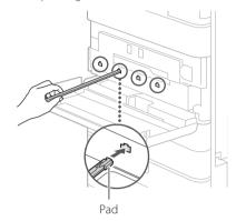
**5.** Insert the cleaning stick in until it hits the bottom of the hole, and gently move it back and forth.
