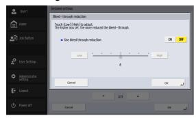
Eliminates bleed-through images, in which images on the reverse side of a scanned document appear on the scanned page, such as when scanning thin documents with text or images on both sides.
