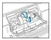
3. Pull the left lever that secures the retard roller to the scanner, and remove the roller.
