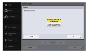
The scanner detects from the scanned image that the document was fed askew and then straightens the image.
