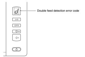
When using the double feed detection ignore function
