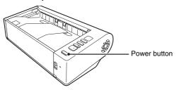
The power button lights blue when the power turns ON.
