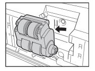
**4** Install the new feed roller, attaching the right side first.
