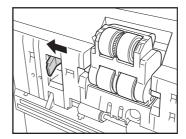
**3** Remove the feed roller, detaching the left side first.
