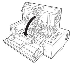
After removing the jammed paper, check to see if the last page was scanned correctly, and then continue scanning.
