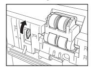
${\bf 2} \ \ \, \overline{ {\rm Slide the securing lever for the feed roller to the left.} }$
