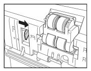
**6** Lower the securing lever for the feed roller until it clicks into place.
