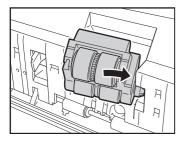
**5** Slide the securing lever for the feed roller to the right.
