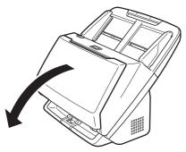
Pull the OPEN lever and pull open the front unit toward you.
