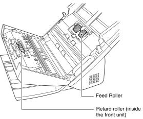
When closing the front unit, make sure that it is completely closed by gently pressing the left and right until you hear a click.
