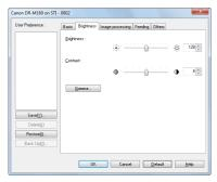
Adjust the brightness and contrast of scanned images. In addition, you can also click [Gamma] and set the gamma correction value for scanned images.
