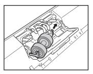
4 Push the left side of the retard roller to secure it to the scanner.
