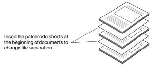
Open the scanner driver settings screen and select [Patchcode] in [Batch Separation] on the [Others] tab.
