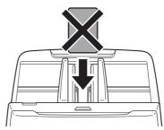
• When scanning cards, clear the [Detect by Ultrasonic] check box in the [Feeding] tab on the scanner driver settings screen. (See p. 28)
