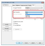
When [Batch Separation] is set to [Auto], the batch is separated after the next document is placed and scanning is continued. For more details about [Blank Page] and [Patchcode], see "Batch Separation" on p. 52
