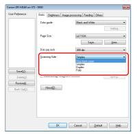
If [Skip Blank Page] is selected, the [Setting] button is enabled, and you can adjust the level for judging whether pages are blank.
