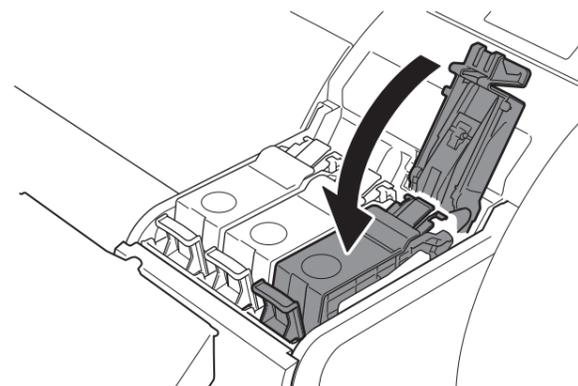
Be sure to look at the labels, and check that the ink tanks are properly installed.
