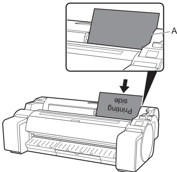
**5** Adjust the position of the width guide (A) according to the size of the loaded paper. Align the width guide exactly with the paper to avoid the loaded paper from tilting or crinkling.
