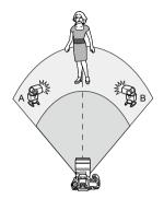
Receivers can be assigned as flash groups A and B, and you can adjust the relative output of each.
