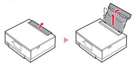
2 Open the feed slot cover and slide the righthand side paper guide to the far right.
