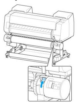
7. Hold roll holder by its flanges (A) and remove from roll holder slot.
