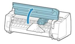
**3.** If the Carriage is out, move the Carriage to the left or right side, away from the jammed paper.
