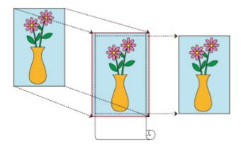
Procedure for printing borderless by enlarging/reducing documents to match roll paper width.
