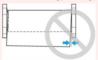
Depending on the paper, the roll paper may be scratched when being fed and not feed well. In this
