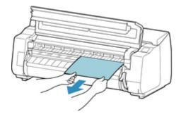
After removing the paper, inspect the interior to ensure paper fragments or other objects do not remain.
