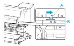
Change Inward/Outward Winding Changeover switch on roll unit to desired winding direction.
