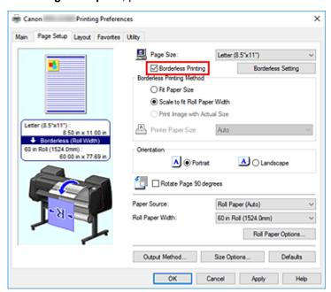
After the **Information** dialog is displayed, under **Roll Width**, select the same paper width as that of the paper roll loaded in the printer and click **OK**.
