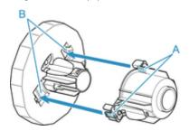
**5.** Insert the holder stopper into the Roll Holder, and then lock it in place.
