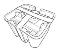
**13.** Remove tape used to secure print head.
