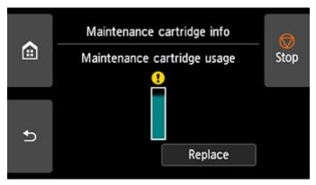
If the touch screen indicates to replace the maintenance cartridge, replace the maintenance cartridge.
