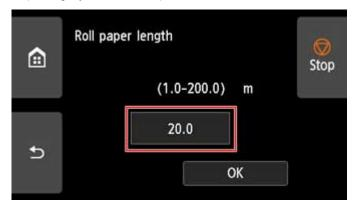
2. Tap the keypad appearing on the touch screen, enter the roll paper length, and then tap **OK**.
