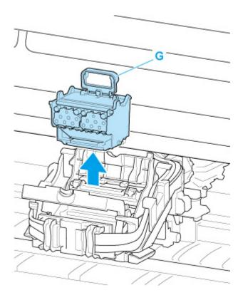
• Never touch the metal contacts of the carriage. Furthermore, do not allow any dirt or debris to become adhered to the metal contacts of the carriage. These may damage the printer.
