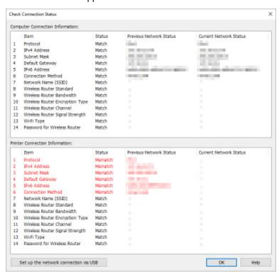
If the network status when you used the printer is different from the current status, **Mismatch** appears on **Status** and the items are displayed in red. Check the red items.
