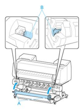
8. Change Roll Holder Lock switch on roll unit to lock direction.
