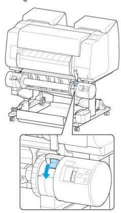
9. Change the feed flap switch on top of the roll unit so that the switch indicator (A) is aligned with ● (B) position on the take-up icon.
