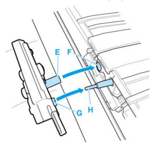
**9.** Install while aligning fixing part included with replacement cutter blade with center of cutter blade.
