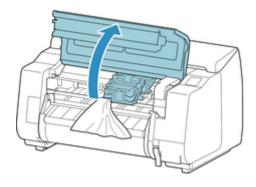
**3.** If the Carriage is out, move the Carriage to the left or right side, away from the jammed paper.
