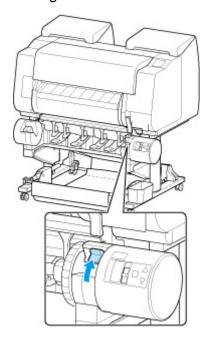
**7.** Hold flanges (A) so that roll holder's black gear is on left, align roll holder shaft with roll holder slot left and right guide grooves (B), and load.
