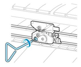
7. Remove cutter blade while holding D.
