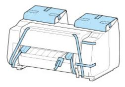
3. If using roll unit, refer to Setup Guide provided with roll unit and attach roll unit to Stand.
