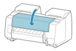
**5.** Tape down printer covers to secure them, in the reverse order of tape removal during installation.
