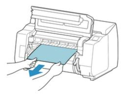
After removing the paper, inspect the interior to ensure paper fragments or other objects do not remain.
