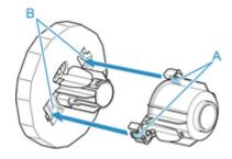
4. Insert paper core, which is for winding roll paper, into roll holder.
