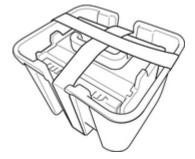
**13.** Remove tape used to secure print head.
