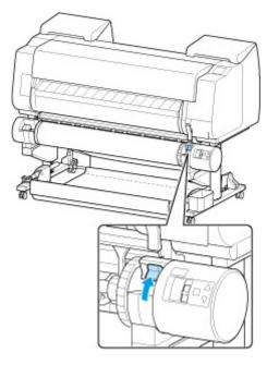
**9.** Hold roll holder by its flanges (A), and remove from roll unit.
