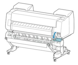
**6.** Hold the used maintenance cartridge by the grip (B) with one hand and put your other hand under the maintenance cartridge to hold it firmly on the bottom, keeping it level as you pull it out.
