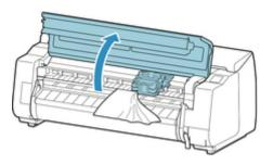
**3.** If the Carriage is out, move the Carriage to the left or right side, away from the jammed paper.
