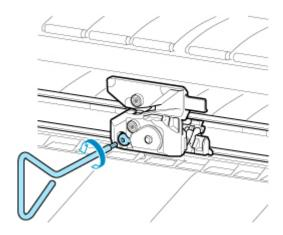
7. Remove cutter blade while holding D.
