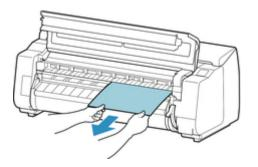
After removing the paper, inspect the interior to ensure paper fragments or other objects do not remain.
