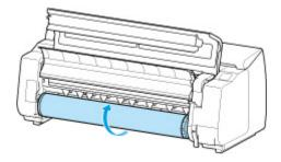
7. Hold Roll Holder by its flanges (A) and remove from roll holder slot.
