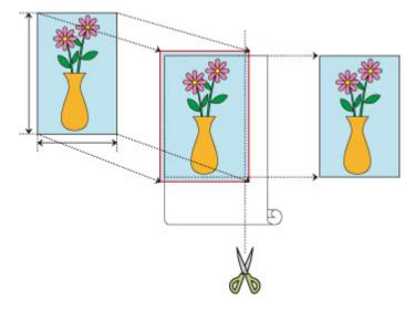
In normal borderless printing, paper sizes that match the width of the roll paper are combined to print without borders on all four sides.
