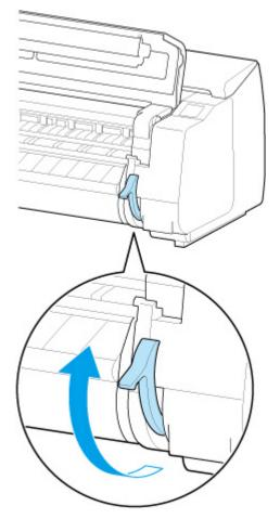
4. Load paper keeping right edge of paper aligned with extended line of paper alignment line (A) on right side of printer and position from which to start printing aligned with groove (B) at far end of platen.
