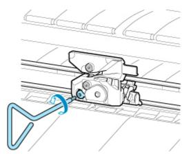
7. Remove cutter blade while holding D.
