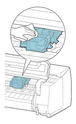
• Do not touch the linear scale (A), carriage shaft (B), or ink tube stabilizer (C). Touching these may cause malfunction.
