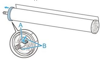
11. Remove printed material that has been taken up, from roll holder for each paper core.
