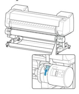
7. Hold roll holder by its flanges (A) and remove from roll holder slot.
