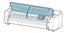
**7.** If the print head locking cover and print head lock lever are dirty, use a damp cloth that you have wrung out completely to wipe them clean.
