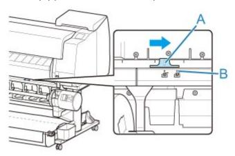
Change Inward/Outward Winding Changeover switch on roll unit to desired winding direction.
