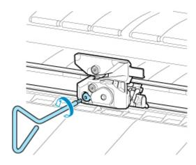
7. Remove cutter blade while holding D.
