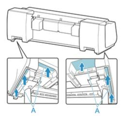
**2.** Remove tape and packaging material attached to the printer. Also open the top cover and remove stoppers and spacers inside the printer.
