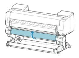
**6.** Change **Roll Holder Lock** switch on roll unit to release position.
