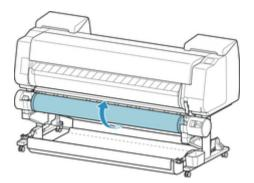
Apply adhesive tape to the rewound paper to hold it in place, if necessary.
