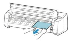
After removing the paper, inspect the interior to ensure paper fragments or other objects do not remain.
