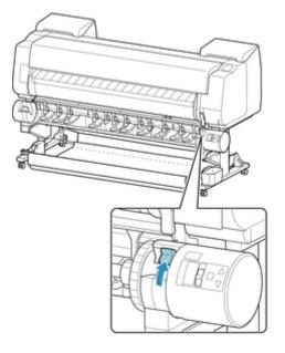
**3.** Hold flanges (A) so that roll holder's black gear is on left, align roll holder shaft with roll holder slot left and right guide grooves (B), and load.
