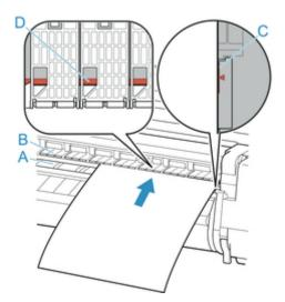
When you insert the sheet, it will adhere automatically to the surface of the platen.
