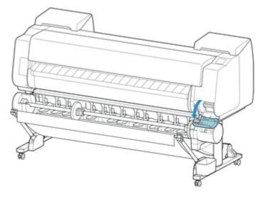
**6.** Hold the used maintenance cartridge by the grip (B) with one hand and put your other hand under the maintenance cartridge to hold it firmly on the bottom, keeping it level as you pull it out.
