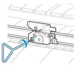
7. Remove cutter blade while holding D.
