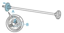
**3.** If taking up roll paper whose paper core has an inner diameter of 3 inches (76.2 mm), insert 3-Inch Paper Core Attachment in roll holder and holder stopper.
