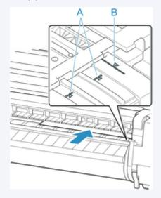
• You can adjust the vacuum strength holding the paper against the platen when the release lever is up. If it is difficult to load the paper, tap **Suction** on the touch screen and adjust the vacuum strength. You can adjust the vacuum strength to 5 levels.
