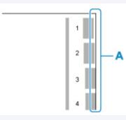
Check the edges (A) of the paper of No. 1 to No. 8 of the output pattern, and select the appropriate number for the amount of protrusion of the printed pattern.
