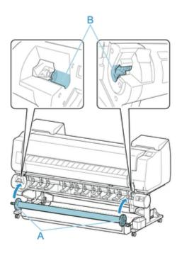
8. Change Roll Holder Lock switch on roll unit to lock direction.
