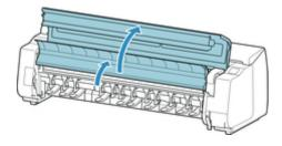
**3.** Hold flanges (A) so that roll holder's black gear is on left, align roll holder shaft with roll holder slot left and right guide grooves (B), and load.
