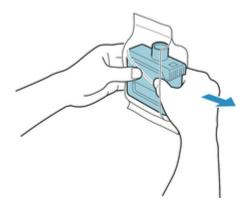
• Never touch the ink holes (D) or the metal contacts (E). This may cause stains, damage the ink tank, and affect printing quality.
