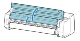
6. Using both hands, rotate the Roll Holder in the direction of the arrow to rewind the roll.
