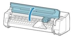
**3.** If the Carriage is out, move the Carriage to the left or right side, away from the jammed paper.
