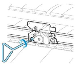
7. Remove cutter blade while holding D.
