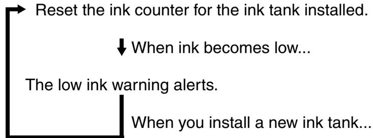
When you reset the ink counter, the counter will assume that the ink tank is full, regardless of how much ink actually remains. Resetting the counter on a *new* ink tank is the only way to match the counter value with the actual ink volume, so you should only enable the low ink warning and reset the ink counter when installing a new ink tank.
