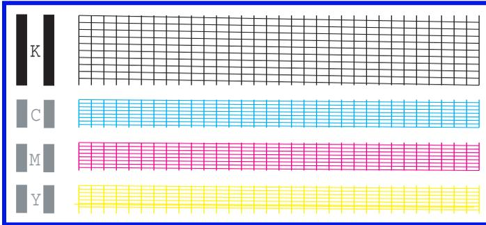
Lines missing indicate the print head requires cleaning.
