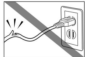
Never plug the printer into a power socket that is shared with other equipment (extension cord, double adapter, etc.).
