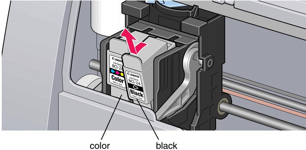
Lift the ink tank from its slot.
