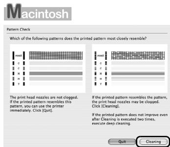
To proceed to cleaning of the Print Head, go to step 4-(3) of the Windows or Macintosh Print Head Cleaning procedure, depending on your platform. See “Print Head Cleaning” on page 35.
