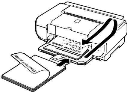
**4** In the printer driver, select **Front Feeder** for **Paper Source**.
