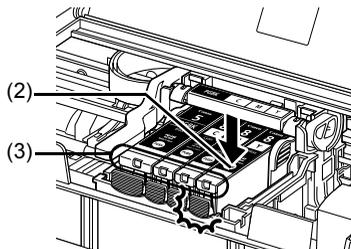
\*1 Make sure the position of the tank matches the label.
