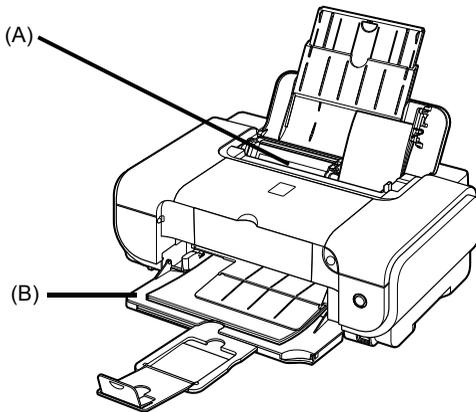
(A) Auto Sheet Feeder: Load paper of various types and sizes, including photo paper
