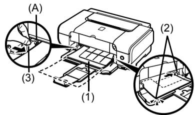
Do not load higher than the Load Limit Mark (A).
