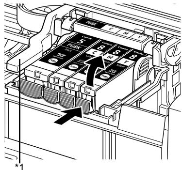
\*1 Do NOT touch the Print Head Lock Lever; remove only the ink tank.
