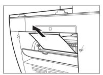
**8** For paper jammed in the paper cassette, pull out the cassette first. Pull down the paper out of the machine.
