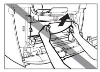
**6** Gently pull jammed paper between output rollers until the leading edge appears.
