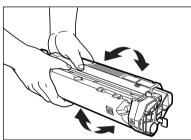
Hold the cartridge. Break the tab (A) and pull out the seal (B) completely.
