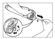
4 Maintenance 17 6 Hold the cartridge and align the projections (A) on the both sides of the cartridge to the guides (B) in the machine, then gently slide the cartridge into the machine as far as it will go.
